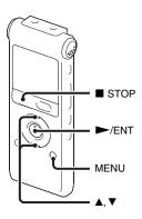
You need to set the clock to use the alarm function or record the date and time. Clock setting display appears when you insert battery for the first time, or when you insert a battery after the IC recorder has been without battery for more than 3 minutes, "Set Date&Time" appears, and then the year section flashes in the display window.
